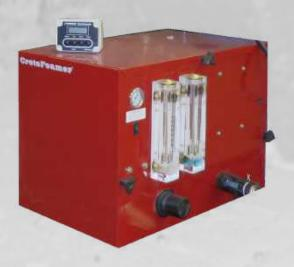
Richway's CFVT-20C is designed as a truck mounted system for either a ready-mix or volumetric truck for the production of cellular concrete. Its compact design utilizes an outside fresh-water and air source. Patented VersaTrac Technology allows foam density, and output adjustment on the job site to meet any specifications. With a foam production output of up to 20CFM (566 L per min) it's an ideal machine for small to medium sized cellular concrete projects.
