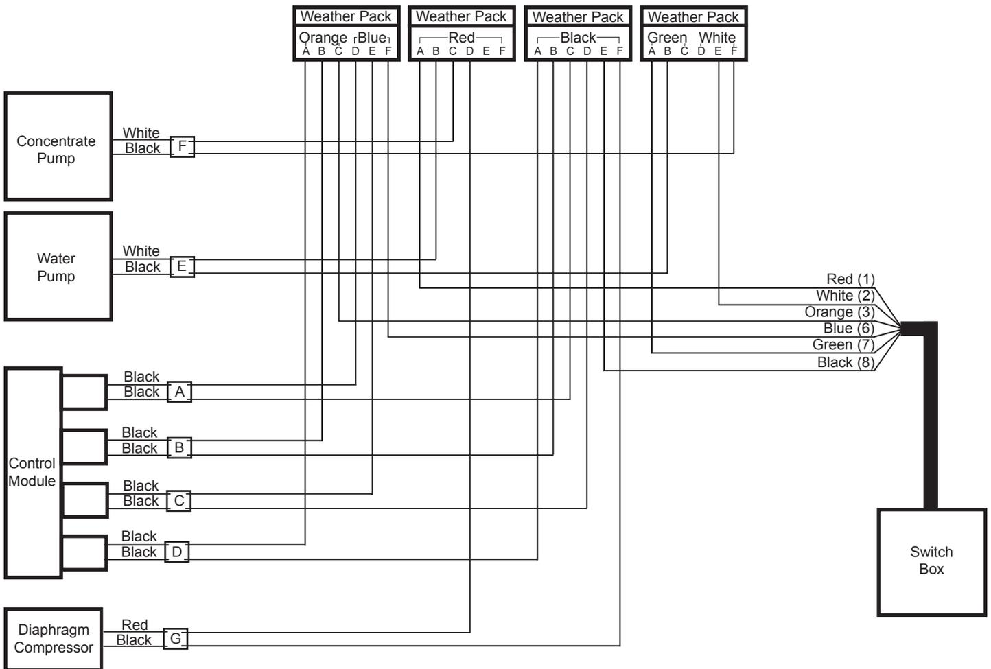
FIGURE 11 - Versa Trac Power Unit Wiring Diagram
