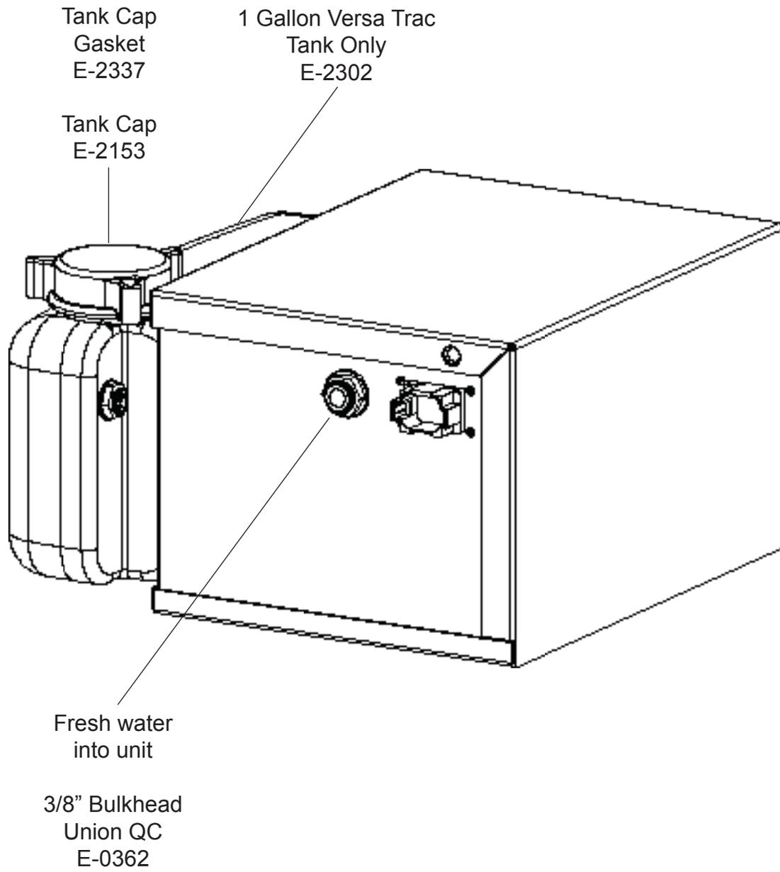
FIGURE 7 - Versa Trac Power Unit External Components
