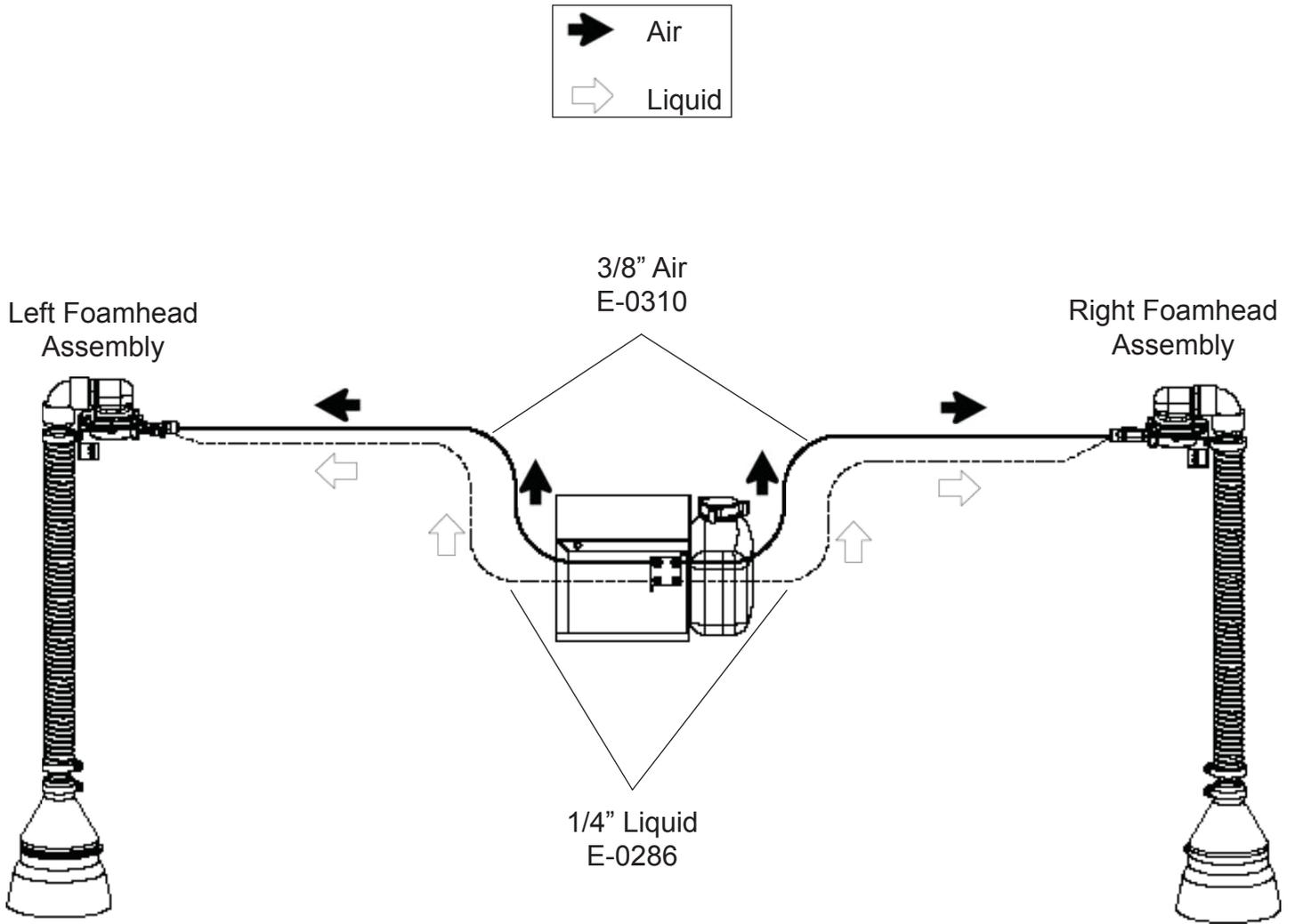
FIGURE 4 - Versa Trac Liquid and Air Flow
