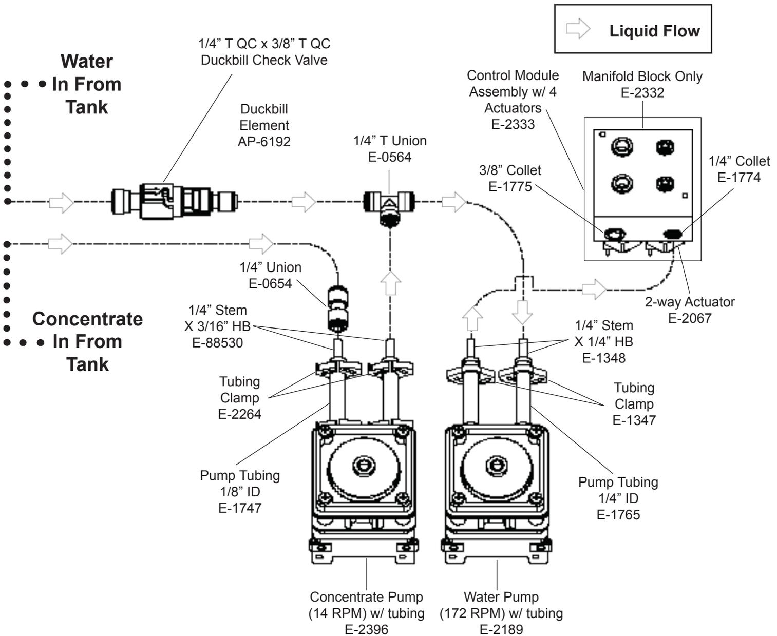
FIGURE 8 - Versa Trac Power Unit Internal Liquid Components
