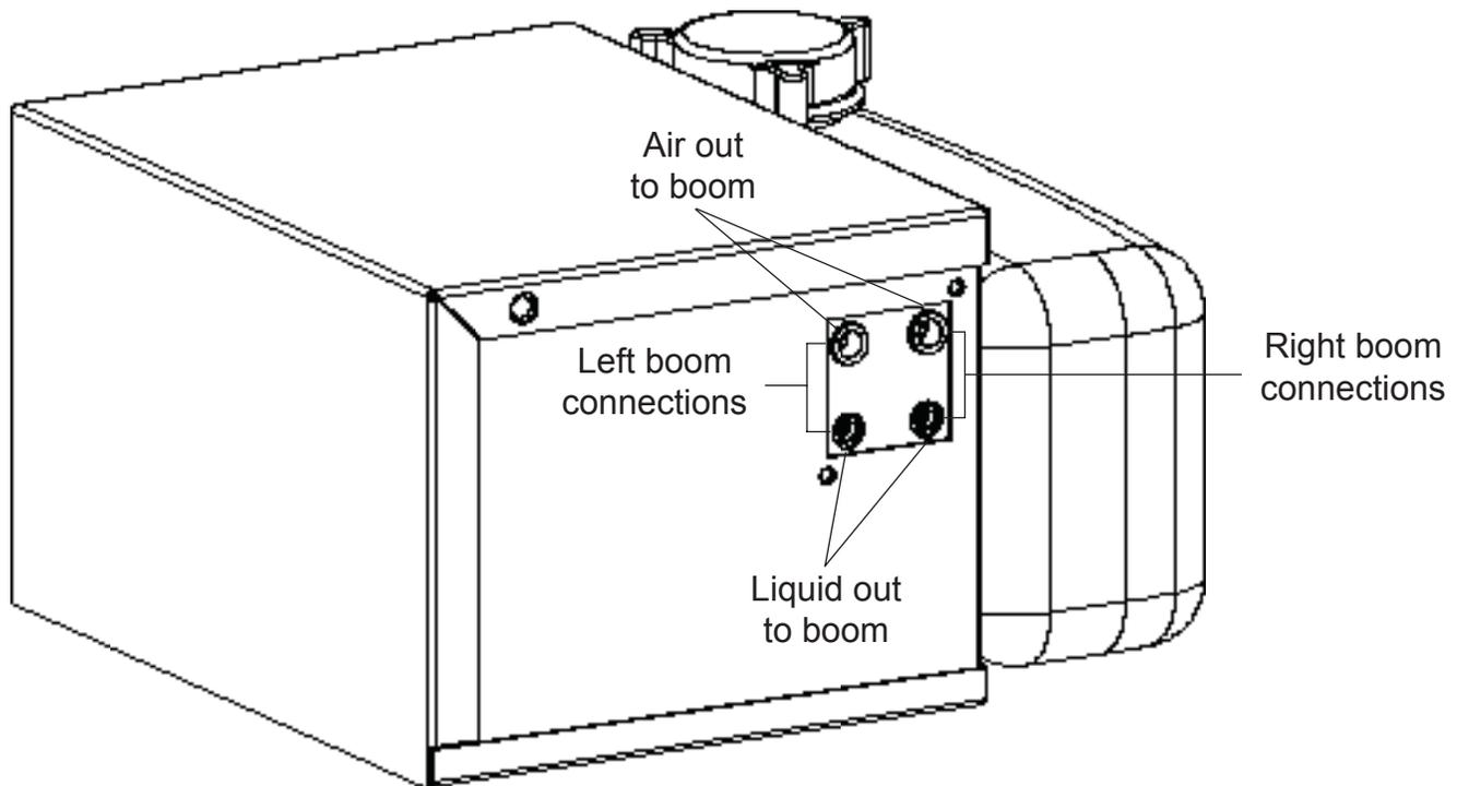
FIGURE 6 - Versa Trac Air/Liquid Connections
