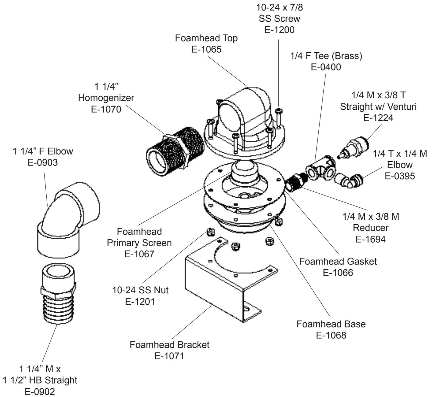
FIGURE 3 - Versa Trac Foamhead Assembly
